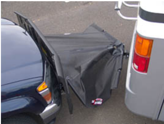
Gas struts allow for cornering without causing damage to the Tow Defender, motorhome or towed vehicle.
